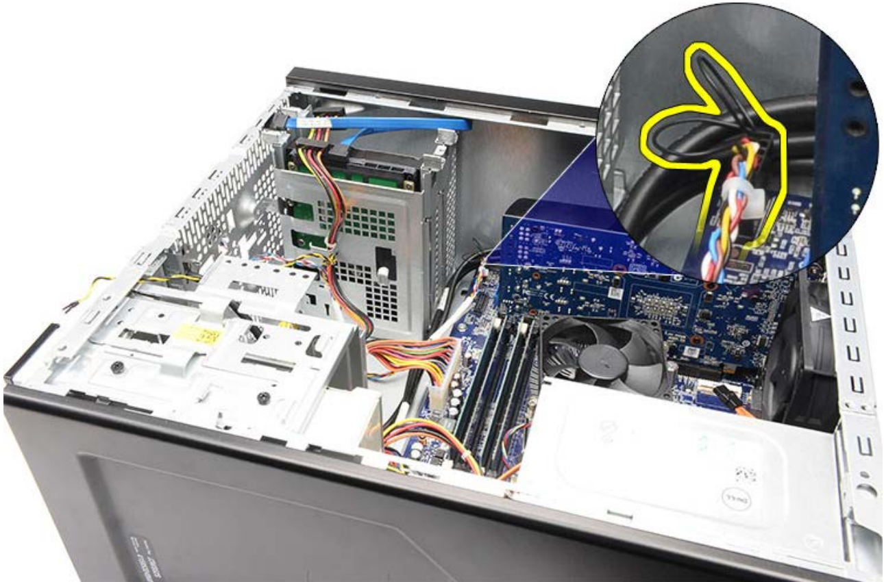
8. Unthread the power button cable from the routing clips.
