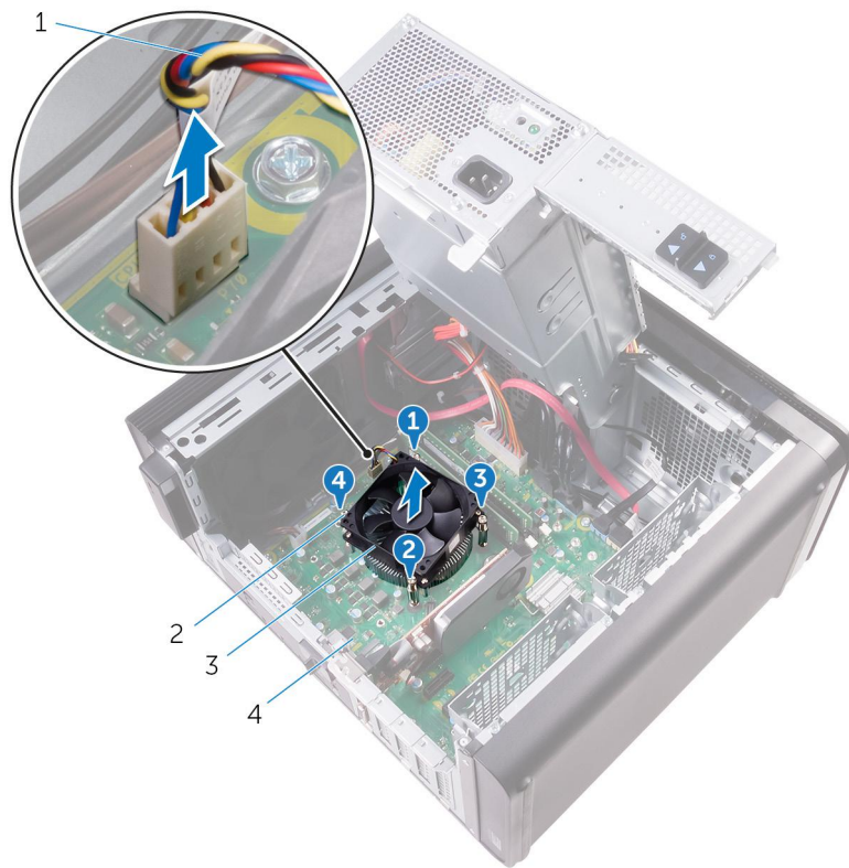
Figure 35. Removing the processor fan and heat sink
