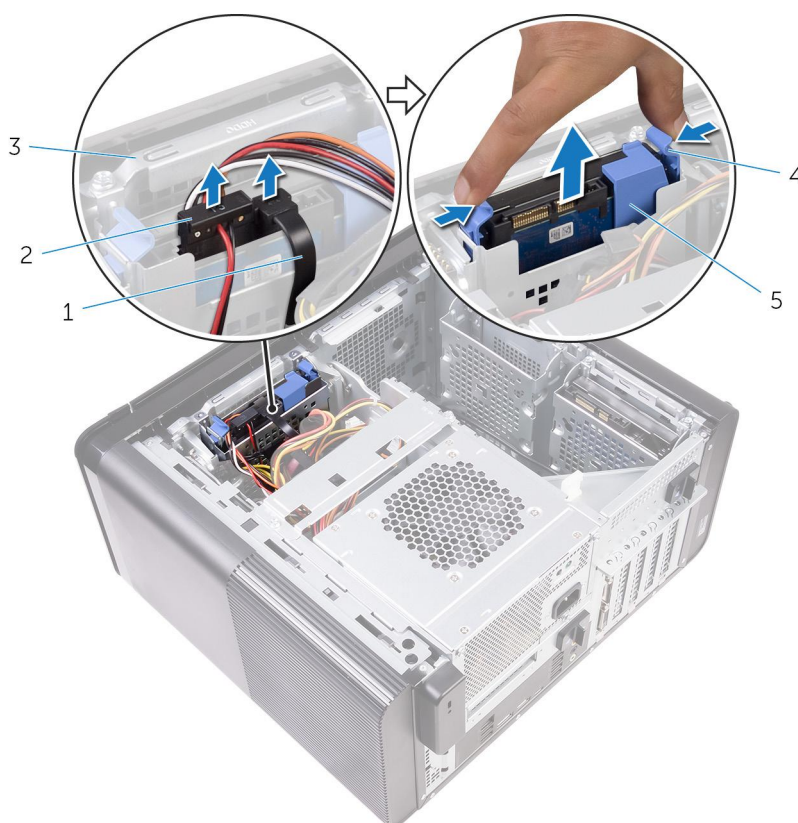
Figure 12. Removing the hard-drive assembly
