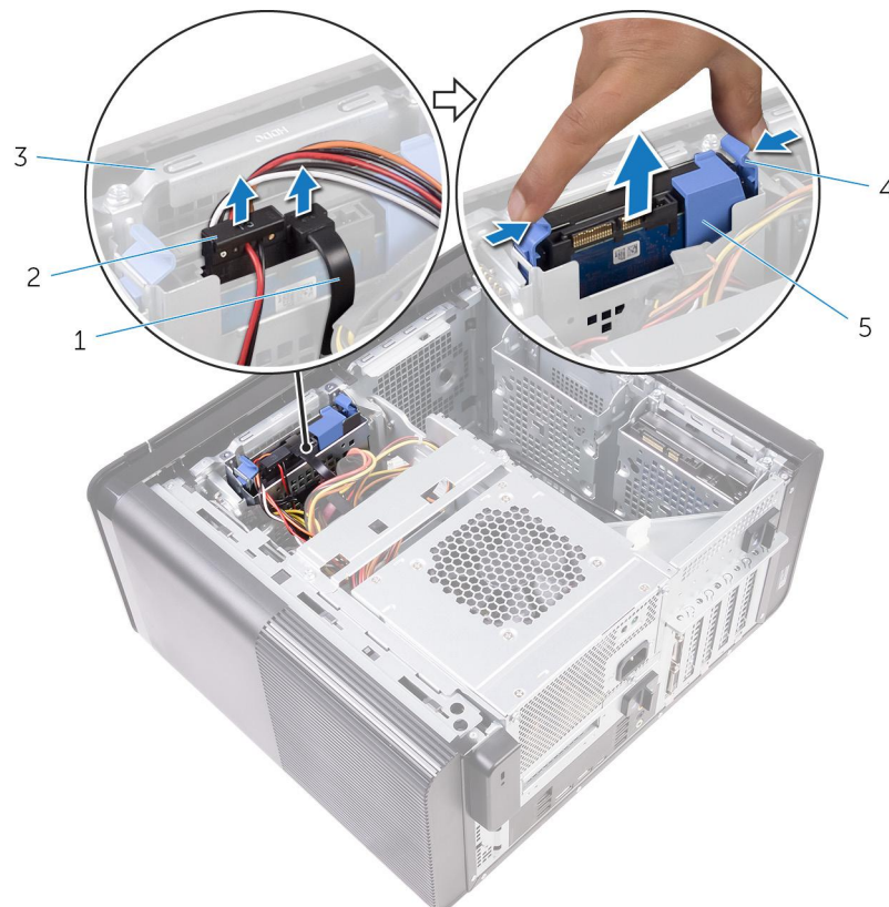
Figure 13. Removing the hard-drive assembly
