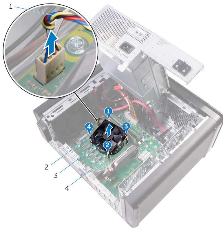
Figure 33. Removing the processor fan and heat sink
