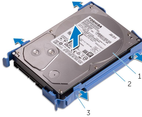
Figure 14. Removing the hard drive from the bracket
