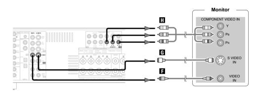
• The component video input and/or output terminals may be labelled differently on some monitors or video components. Check the owner's manuals for other components for further information.
