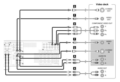
• When recording to a VCR, it is necessary that the type of cable used with the playback source equipment be the same type that is connected to the AVR-1507 VCR OUT terminal.
