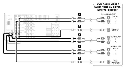
• With discs on which special copyright protection measures have been taken, however, the digital signals may not be output from the DVD player. In this case, connect the DVD player's analog multi-channel output to the AVR-1507's EXT. IN terminals for playback. Also refer to your DVD player's operating instructions.
