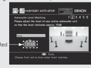
\* If the measured level is outside the 72 ~ 78 dB range, the level indicator is red.
