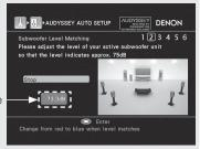
\* If the measured level is within the 72 ~ 78 dB range, the level indicator is blue
