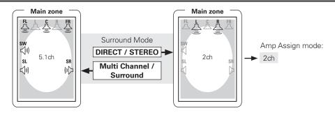
☐ Amp Assign mode setting and speakers connected to the various speaker terminals
