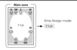
☐ Amp Assign mode setting and speakers connected to the various speaker terminals
