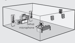
It is not recommended to hold it in your hand. Be sure that the path from microphone to the speakers is not blocked by objects. Avoid placing the microphone close to a seat back or wall as sound reflections may give inaccurate results.
