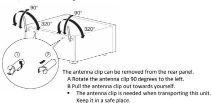
Attach the antenna clip by following the steps for removing it in reverse.
