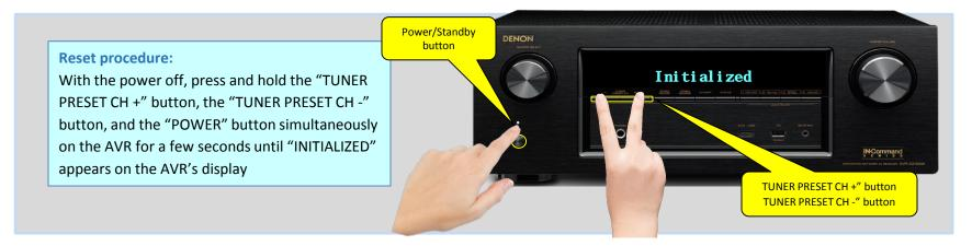
Resetting the micro is a procedure used to "reboot" the microprocessor to restore its normal operation when it temporarily freezes, locks up, or behaves erratically. Resetting the microprocessor, erases any saved settings you may have previously programmed into the unit
