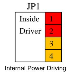
**【Notice】** When the initial electric current of the lock is less than 500mA/12V, you can access to the internal driven mode and use the POE of the Voice Access System or 12V DC to control the the switch of the electric lock ; When the initial electric current of the lock is more than 500mA/12V, you need to access to the external driven mode(Use specialized DC power to control the electric lock )
