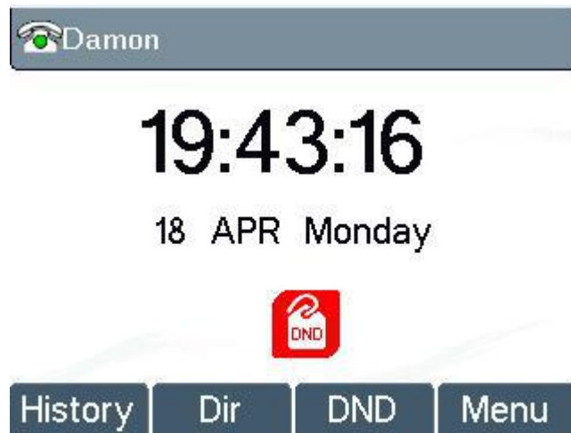
Figure 57 - DND Enabled on All Lines
