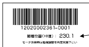
Figure 4.4-1 Magnetic Pole Position Offset Label Attaching Position Examples
