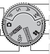
**P, S, A, M**: Select for full control over camera settings, including aperture (**M** and **A**) and/or shutter speed (**M** and **S**; pg. 40).
