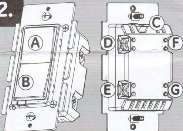
**A. Top Rocker** — [Press & release to turn fan control on, press & hold increases speed]
