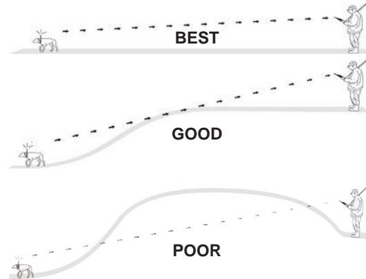
Line-of-Sight Radio Communication
