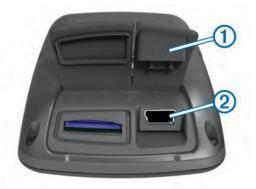
2 Plug the small end of the USB cable into the mini-USB port.
