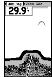
Structure is soft, probably a mud pile
