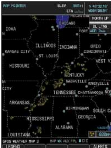
Figure 4-100 GFDSD Data Link Lightning and Legend
