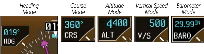
Figure 1-16 Selection Modes Adjusted with the PFD Knob
