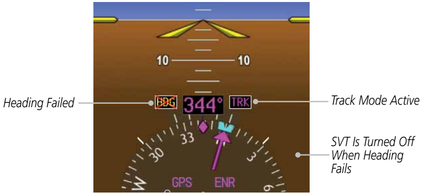
Figure 1-13 Track Mode shown as Active when Heading Info has failed
