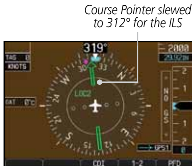
Figure 2-34 Auto-Slewing HSI with ILS Loaded and Shown with the Corresponding Approach Plate
