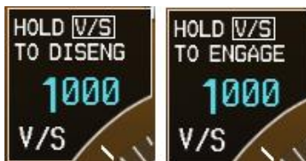
Figure 5-34 Pressing and Holding the VS Key to Engage/Disengage VS mode
