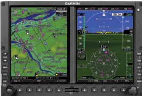
Figure 1-3 GDU 620 PFD and MFD with PFD on Right
