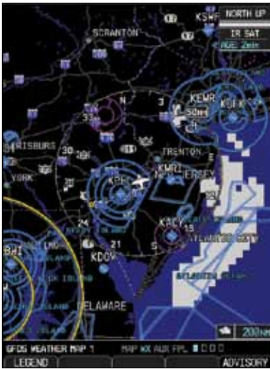
Figure 4-98 GFDS Infrared Satellite Data Map Display and Legend
