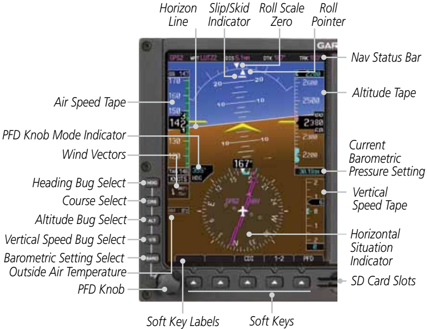
Figure 2-1 PFD Description (Ground Pointer Mode)
