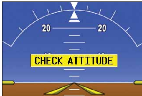
Figure 5-27 Check Attitude - Autopilot Automatically Disconnected
