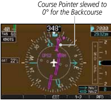
Figure 2-35 Auto-Slewing HSI with Localizer Backcourse Loaded and Shown with the Corresponding Approach Plate
