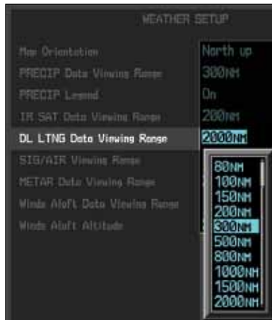
Figure 4-101 GFDS Lightning Viewing Range Selection
