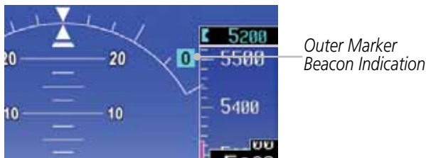
Figure 2-42 Marker Beacon Location
