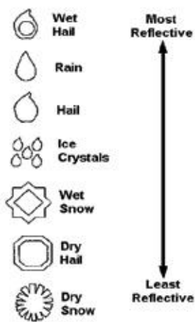
Figure 4-58 Precipitation Type and Reflectivity
