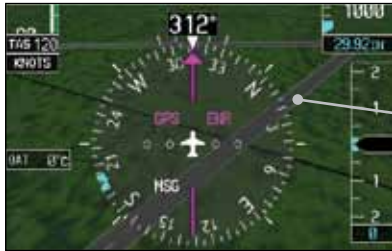
Figure 5-43 Depiction of Runway with a Loaded Flight plan
