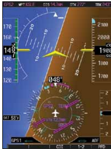
Figure 2-19 Extreme Roll Indication with Display Declutter
