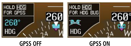
Figure 5-31 GPSS mode control with the HDG key
