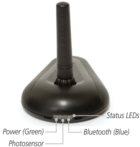
Figure 4-2 GDL 39 Status LEDs
