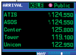
Press ENT to show the frequencies for the selected airport.
