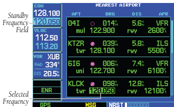
Figure 8-7 Frequency Moved to Standby Field
