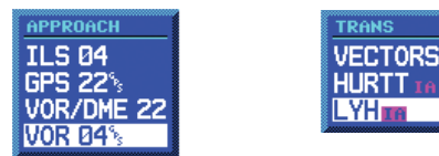
Figure 6-11 Approach and Transitions Windows
