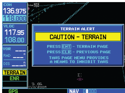
Figure 13-3 Caution Alert Pop-up
