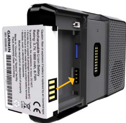
Installing the Battery
