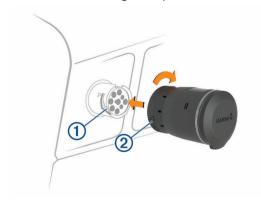
3 Turn the lock ring clockwise until it locks into the diagnostic port.
