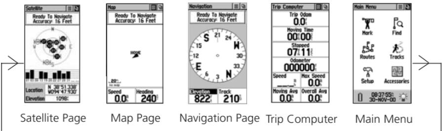
While these five pages provide you with different types of navigation information, they all share common features like Option Menus and a Main Page Menu, both of which are accessed by on-screen buttons. To display these menus, simply highlight the on-screen button and press in on the **CLICK STICK**.
