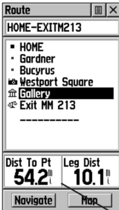
Distance to Point vs Leg Distance. To view Leg information, highlight the end waypoint on a leg.
