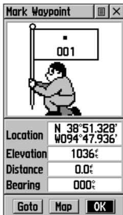
The Mark Waypoint Page displays your Marked Waypoint, along with the latitude and longitude and approx. elevation. On-screen buttons can create a Direct path (Goto) to the waypoint, show it on the map (Map), and confirm your selection as a waypoint (OK).
