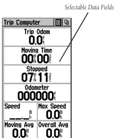
The Trip Computer page displays up to eight different types of navigation data. Each data field is selectable and can contain one of many data information options.
