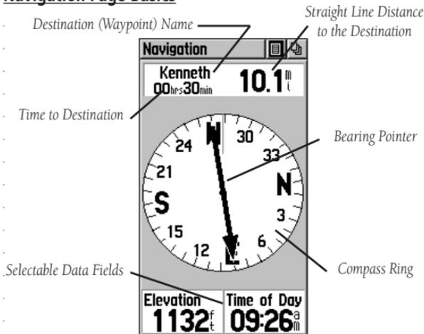
The Navigation Page displays directional information to guide you to a destination. The Status Window at the top of the page shows you the name of your destination, the distance and the time to go. A Bearing Pointer and Compass Ring are displayed to provide you with navigational guidance. Two Data Fields are provided, and can be programmed to display a variety of navigation data.
