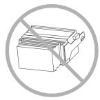
The battery pack must remain in an upright position.
