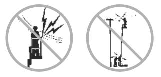
Keep away from the machine if it contacts energized power lines or becomes electrically charged. Personnel on the ground or in the platform must not touch or operate the machine until energized power lines are shut off.
