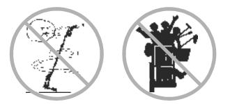
Occupants, equipment and material shall not exceed the maximum platform capacity.
