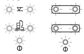
Note: Two different interlock display decals were produced. The symbols on them are different but they both operate the same way. Both are illustrated in this text.
