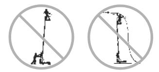
Do not cause a horizontal force or side load to the machine by raising or lowering a fixed or overhanging load.
