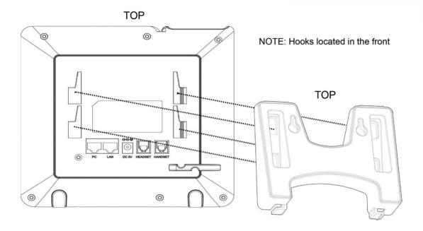
Figure 3: GXP16xx Wall Mount installation
