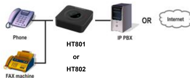
Figure 5: Connecting the HT801/HT802
