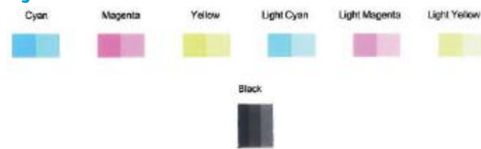
Figure 8-2 Example of color blocks with defects
