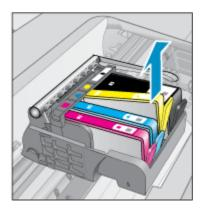
4. Hold the ink cartridge by its sides with the bottom pointing up and locate the electrical contacts on the ink cartridge. The electrical contacts are four small rectangles of copper or gold-colored metal on the bottom of the ink cartridge.
