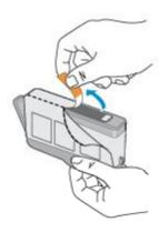
**b**. Twist orange cap to snap it off. A forceful twist may be required to remove cap.
