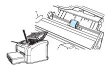
4 Release the small, white tabs on either side of the pickup roller, and rotate the pickup roller toward the front.
