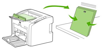
5. Place the pages from side one back in the input tray. Side one should be facing down with the bottom edge feeding into the printer first.
