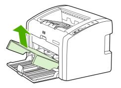
2. Before loading the envelopes, slide the media guides outward to slightly wider than the envelopes.
