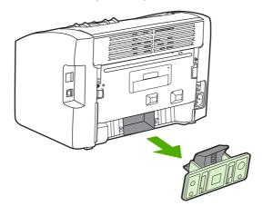
4. Insert the new separation pad, and screw it into place.
