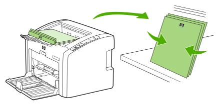
5. Place the stack back in the input tray. Side one should be facing down with the bottom edge feeding into the printer first. Replace the media input tray cover.
