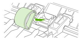
6. Position the new pickup roller in the slot. The circular and rectangular slots on each side will prevent you from installing the roller incorrectly.
