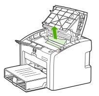
3. When you have removed the jammed media, replace the print cartridge, and close the print cartridge door.
