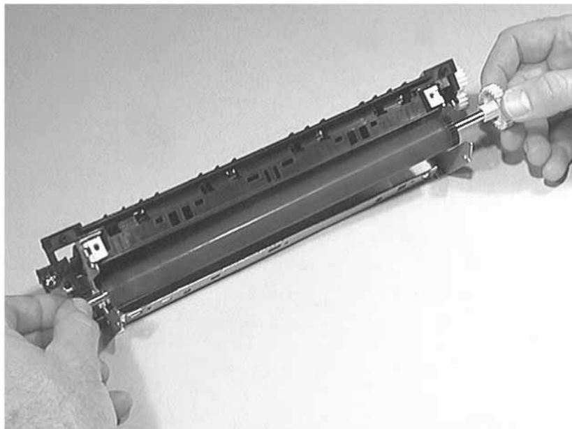
Figure 7-46 Removing the Pressure Roller
