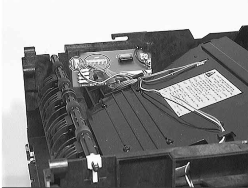
Figure 7-96 Disconnecting Laser Scanner's and Fan's Power Cable
