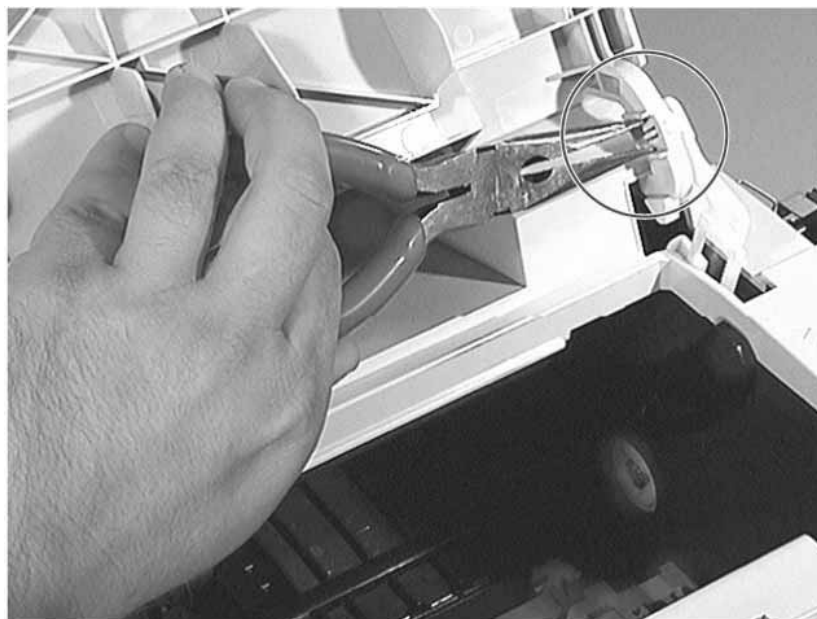
Figure 7-51 Releasing Swing Arm from Toner Cartridge Door
