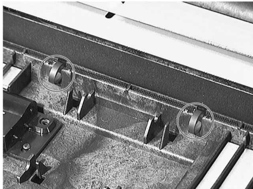
Figure 7-67 Installing the A-1 Belt and Roller
