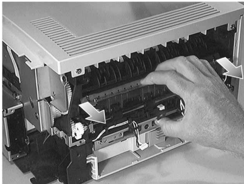
Figure 7-39 Removing the Fusing Assembly
