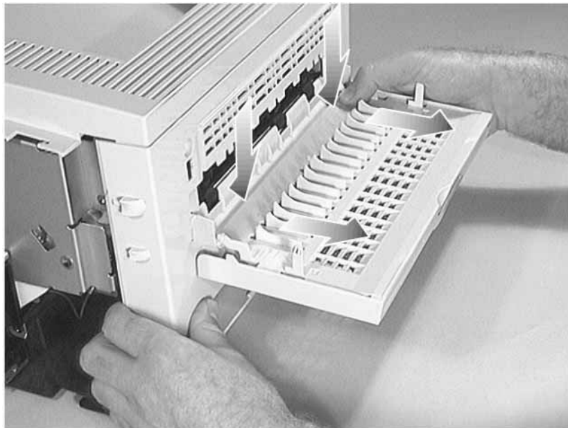
Figure 7-33 Removing the Rear Cover
