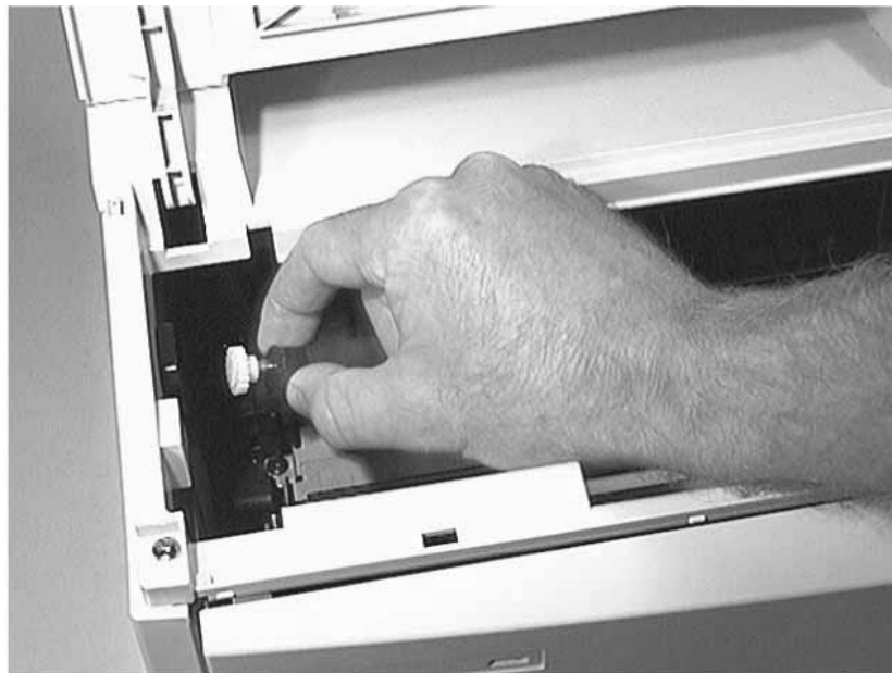
Figure 7-6 Removing the Transfer Roller (2 of 2)
