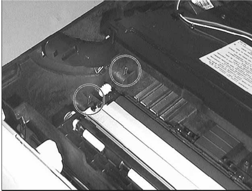
Figure 7-121 DC Bias Voltage Contacts (Leaf Springs)
