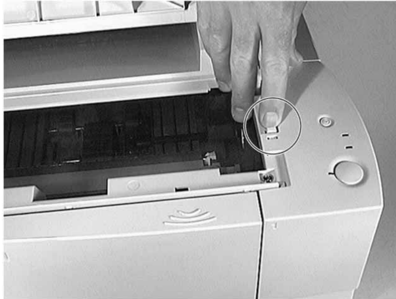
Figure 7-24 DIMM Cover Release Button
