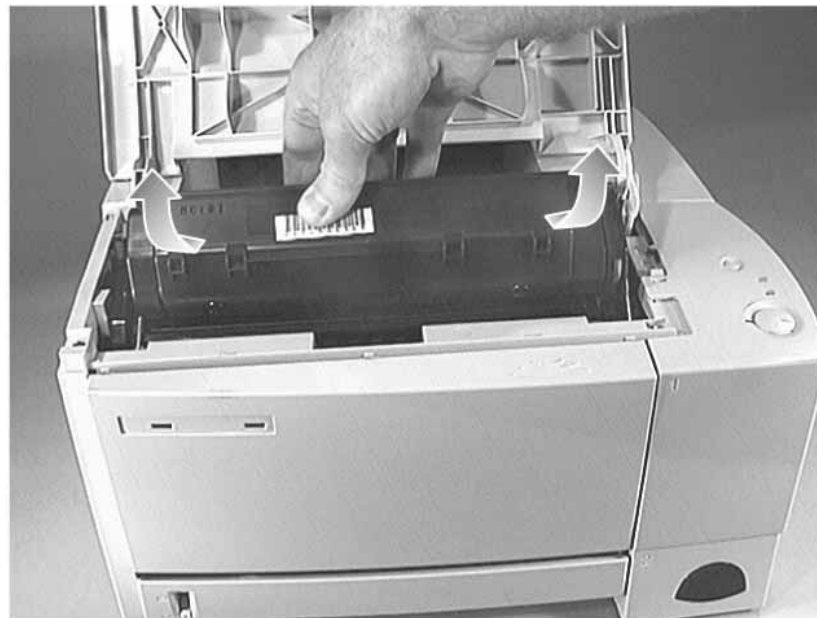
Figure 7-2 Removing the Toner Cartridge
