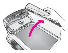
3 Lift the automatic document feeder mechanism.
