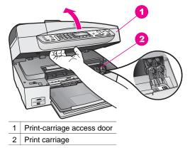
3 Wait until the print carriage is idle and silent, and then lightly press down on a print cartridge to release it.
