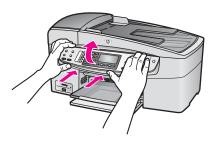
9 Retain the control panel overlay. Do not return the control panel overlay with the HP all-inone.
