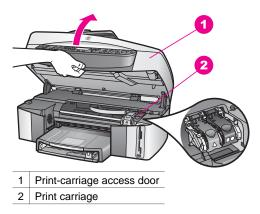
3 When the print carriage is idle and silent, press down and then lift a latch inside the HP all-in-one.
