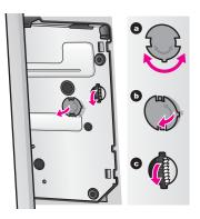
4 Open the print-carriage access door, and then remove the print cartridges from their slots and lower the latches.
