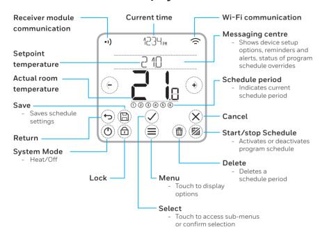
**Note:** To save power, the screen will dim and enter idle mode 45 seconds after the last button touch. The screen will light up when you touch any button.
