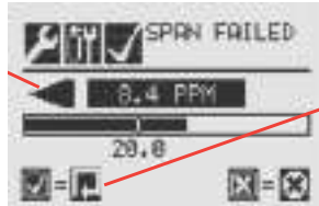
Figure 211. Span Failed screen
