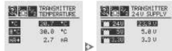
Figure 171. Transmitter Temperature and Supply Voltage Screens
