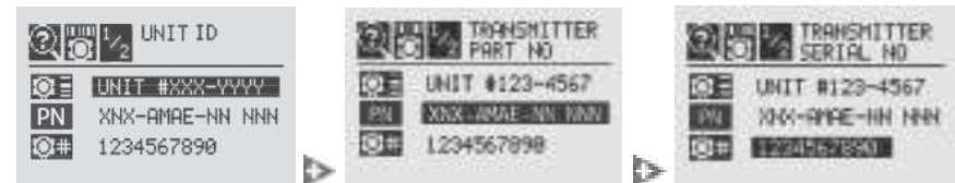
Figure 167. Transmitter ID, Part Number and Serial Number Screens
