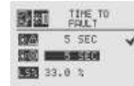
Figure 114. Beam Block Fault Time
