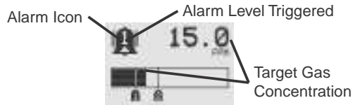
Figure 16. General Status Alarm detail
