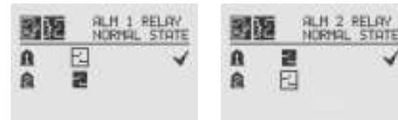
Figure 186. Relay State Screens
