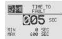
Figure 115. Setting Beam Block Fault Time
