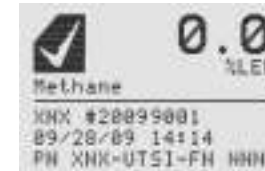
Figure 22. General Status Screen with Unit Information
