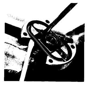
Check the clutch shoes for wear by measuring the material thickness at the shoes thinnest point. If the shoe is worn to less than 1 mm (0.040 in.) of material at the most worn part, the shoes must be exchanged.
