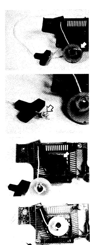
Pull the starter cord up into the pulley notch and rotate the pulley clockwise two turns.
