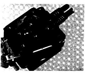
Clean the carburetor body and blow out all passages and channels with low pressure compressed air.
