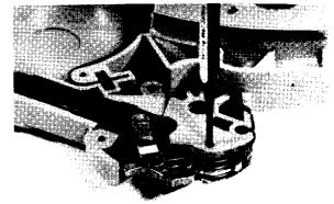
Turn the cover over and press out the brake bank retaining pin with a punch.
