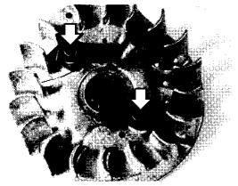
Inspect the starter pawls and springs. Replace components if necessary. Reassemble the pawls and springs in the reverse order of disassembly. Press the pawl retaining pins into the flywheel. Make sure that the shoulder on the pins are flush against the flywheel surface and that the pawls pivot freely.
