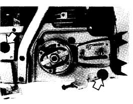
Use a screwdriver to remove the rubber elements.
