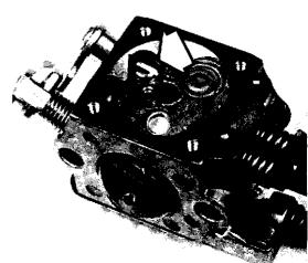
Check the lever. Replace a damaged or worn lever.
