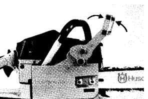
Mount the bar, chain and chain brake to the saw. Before running the saw, check the brake function by moving the hand guard forward until the brake engages. With the brake engaged, it should not be possible to rotate the saw chain around the guide bar. Pull the hand guard back towards the front handle to disengage the brake.
