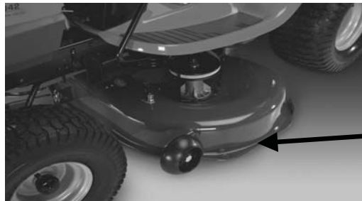
Stamped Deck Shell below, NOT reinforced
