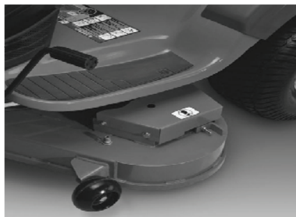
Fabricated Deck Shell Example Below
