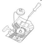
Remove the recoil spring by turning the starter over and loosen the hooks, with the help of a screwdriver. The hooks hold the return spring assembly on the starter.
