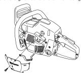
CAUTION! If the special winterising kit has been fitted or any measures have been taken to increase the temperature these changes must be reversed before the machine is used in normal temperature conditions. Otherwise there is a risk of overheating, resulting in severe damage to the engine.
