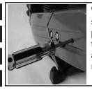
When tightening the hub nut, use a screwdriver to lock the blade shaft in position. Push the screwdriver into the slot (see picture) and rotate the arbor until the screwdriver stops the rotation.
