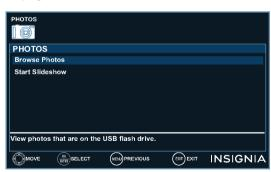
2 Press ▲ or ▼ to highlight Browse Photos, then press ENTER or ▶. The screen displays folder names and photo files stored on the USB flash drive in a thumbnail index with the first folder or file highlighted. A control bar appears at the bottom of the screen.
