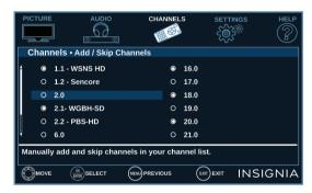
4 Press ▲ ▼ ◄ or ► to highlight the channel you want to hide, then press ENTER. Each channel has a circle to the left. When you hide a channel the circle is empty.
