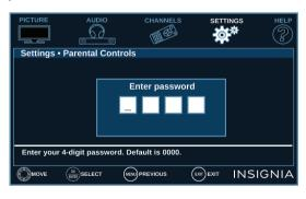
**4** Press the number buttons to enter the four-digit password. The default password is **0000**. You should change the password to a number you can remember
