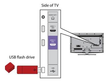
1 Plug a USB flash drive into the **USB** port on the side of your TV.
