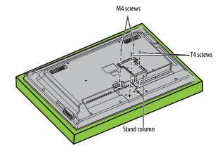
3 Make sure that the wide portion of the stand faces the front of your TV, then align the stand with the stand column and secure the stand to the TV with the four M5 screws provided.
