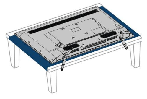
2 If the TV stands are installed, remove the four screws that secure the stands to your TV.
