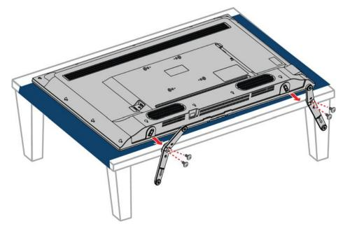
3 Attach the wall-mount bracket to your TV using the mounting holes on the back of your TV. See the instructions that came with the wall-mount bracket for information about which screws to use and how to correctly hang your TV.
