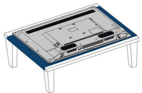
2 Make sure that the arrows on the bottoms of the stands point toward the front of the TV. Align the screw holes on the TV stands with the holes on the bottom of your TV, then secure each stand with two of the provided screws.
