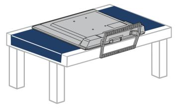
2 If the TV stand is installed, remove the four screws that secure the stand to your TV.
