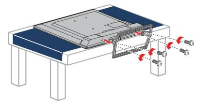
**3** Attach the wall-mount bracket to your TV using the mounting holes on the back of your TV. See the instructions that came with the wall-mount bracket for information about how to correctly hang your TV.
