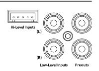
You may run a stereo or a mono signal into the inputs of the amplifier. The amplifier's input section automatically sums stereo signals to mono for the internal amplifier section.
