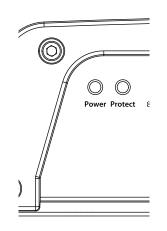
There are two status indicator lights on the amplifier's control panel. These are as follows:
