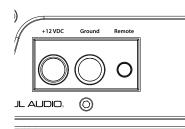
The amplifier will turn on when +12V is present at its **"Remote"** input and turn off when +12V is switched off. If a source unit does not have a dedicated remote turn-on output, the amplifier's turn-on lead can be connected to +12V via a switch that derives power from an ignitionswitched circuit.
