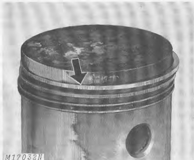
Fig. 11-Scratched Ring Faces Caused by Abrasives in the Engine
