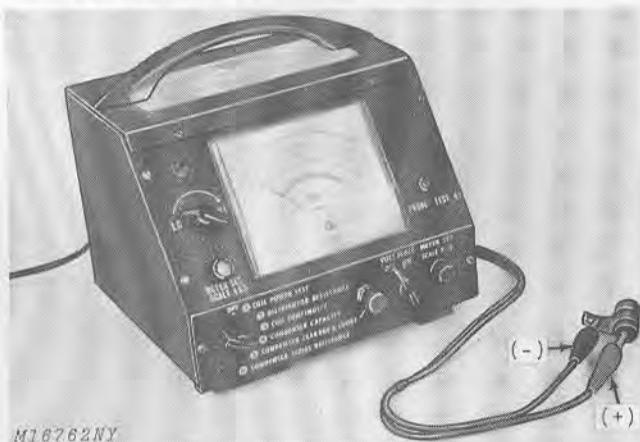
Fig. 16—Testing Condenser Capacity
