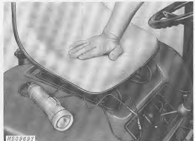
Fig. 8—Testing Seat Safety Switch
