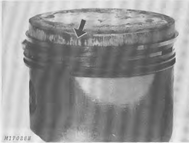
Fig. 7-Scored Piston and Rings
