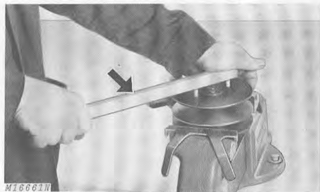
Fig. 18-Removing Variator Sheaves with Special Tool
