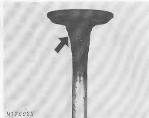
Fig. 5-Lead Deposits on Leaky Intake Valve
