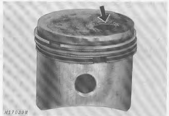
Fig. 18-Hole Burned in Piston Caused by Pre-Ignition
