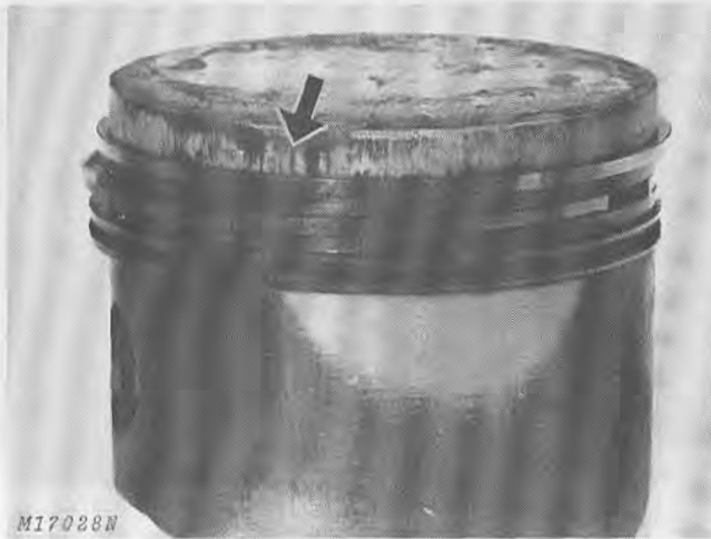
Fig. 7-Scored Piston and Rings
