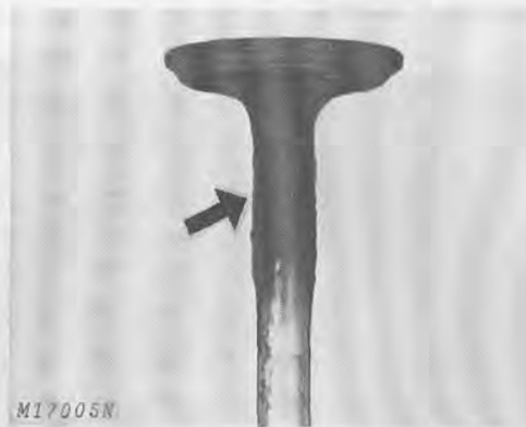
Fig. 8—Gummy Valve Causing Valve to Stick
