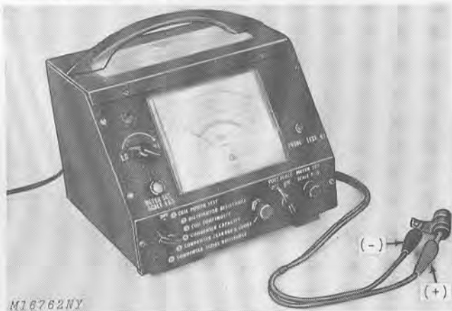
Fig. 16—Testing Condenser Capacity
