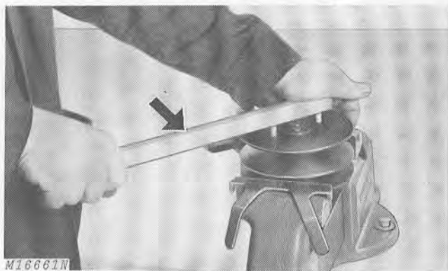
Fig. 18-Removing Variator Sheaves with Special Tool
