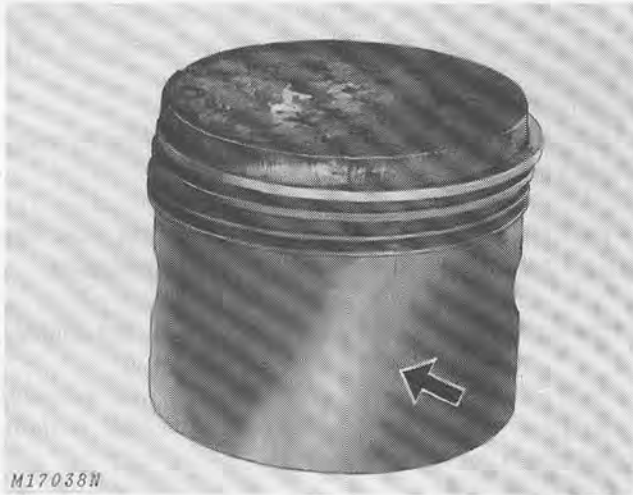
Fig. 17-Diagonal Piston Wear Pattern Caused by Bent or Twisted Connecting Rod
