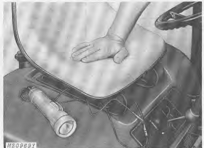
Fig. 8—Testing Seat Safety Switch
