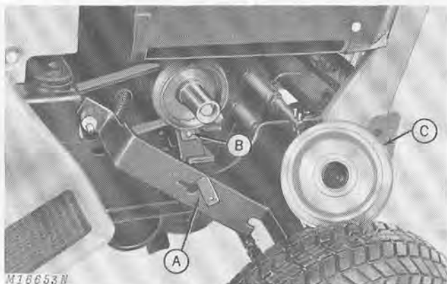
A—PTO Arm B—PTO Brake Shoe C—Clutch Sheave
