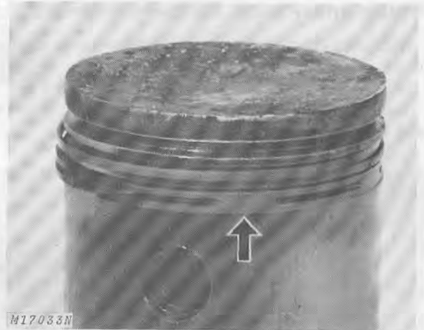
Fig. 12-Worn Oil Rings Which Cannot Provide Oil Control
