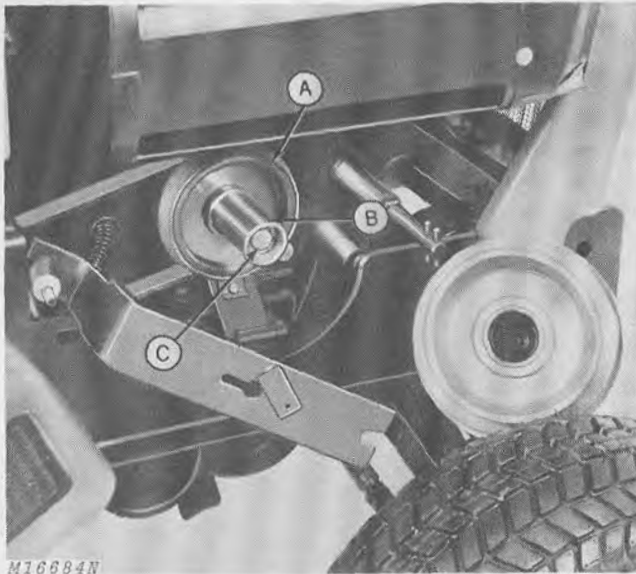
A—Clutch Cone With Brake Lining B—Bearing Inner Race C—Cap Screw
