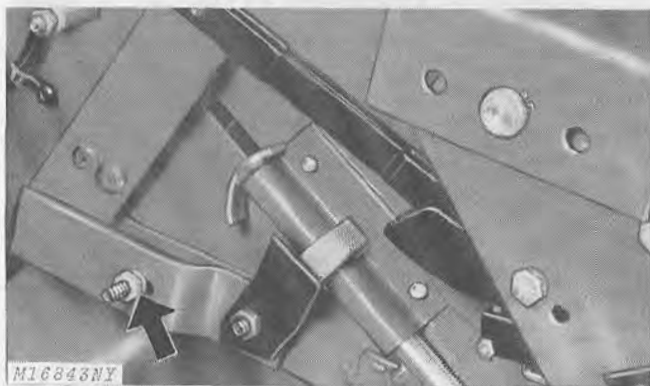
Fig. 10-Adjusting Lift Lever Tension
