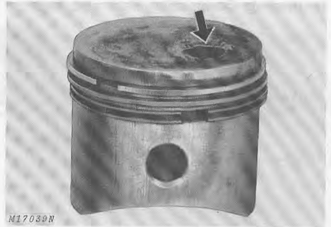
Fig. 18-Hole Burned in Piston Caused by Pre-Ignition
