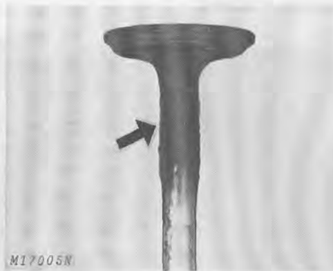
Fig. 8-Gummy Valve Causing Valve to Stick
