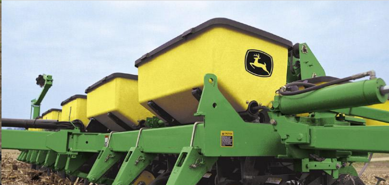
Each fertilizer hopper holds about 550 pounds of dry fertilizer for longer running intervals. The lid opens wide for fast filling, and the entire hopper pivots for easy dumping. Available on 1750, 1770, and 1780 Planters. Drives and transmissions are included.
