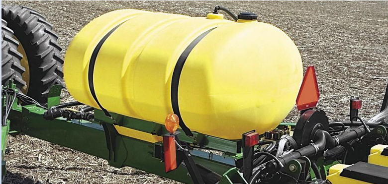
A centrally-located 600 U.S. gallon fertilizer tank is available for the 16-row and 24-row 1770NT Planter. A 420 U.S. gallon frame-mounted fertilizer tank is offered with the 30-foot 1790 Planter. Other tank options are available for additional planter models; see your dealer for more information.
