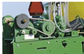
This single-piston, variable-stroke pump uniformly applies liquid fertilizer. Positive displacement produces delivery rates of 1.9 to 38 US gallons per acre. Application rates aren't ground-speed dependent.
